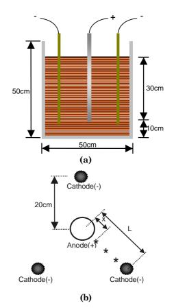
Figure 2. Model (a) and Configuration (b) of The Electrodes in The Soil Sample
